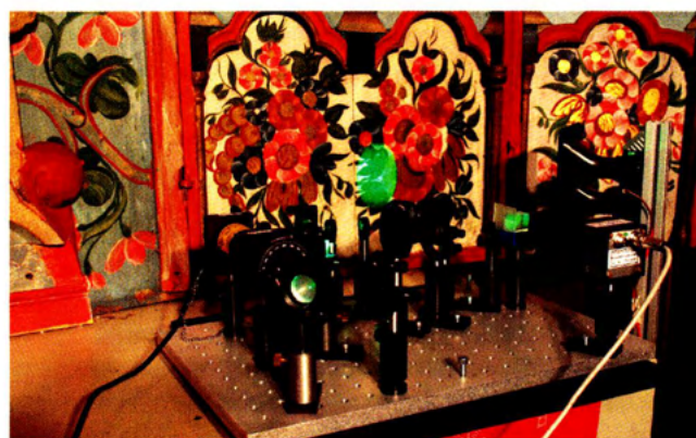
Fig. 20 - DSPI system on the altar during the measurements - the field illuminated by a laser beam is visible.
