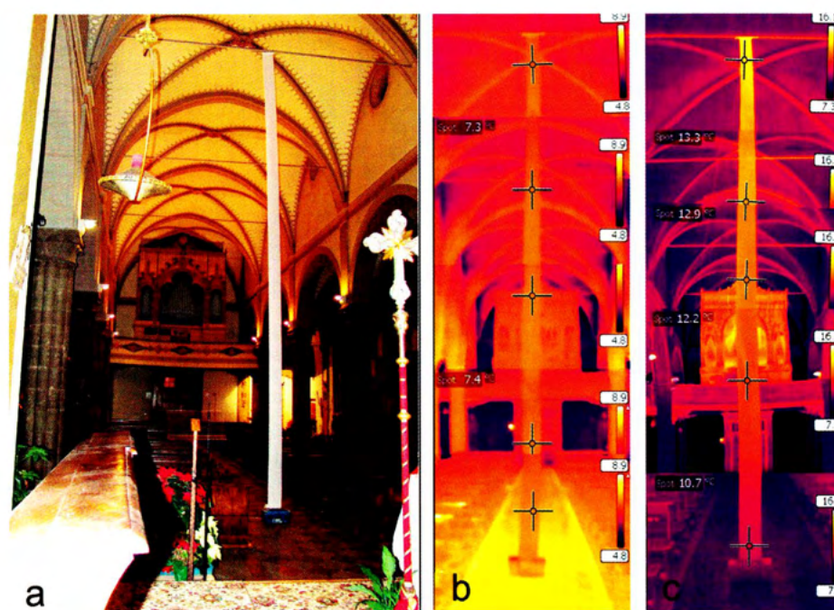
Fig.9 - Visible (a) and infrared (b,c) pictures of the rear part of the church with the organ and the blackbody strip from the floor to the ceiling made with white paper roll. Figures b and c at mid heating and after one hour operation, respectively. In (c) the paper strip shows a clear thermal layering. The organ temperature follows closely the air temperature.
