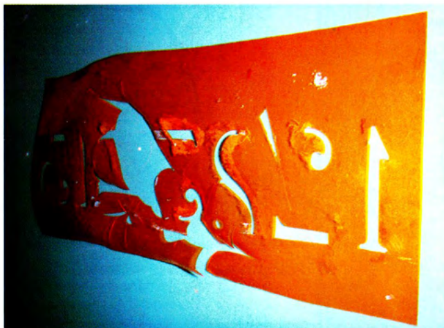
Fig. 12 - Damaged cellulose acetate plotting sheet.
