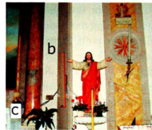
Fig.5 - (a) Infrared picture of a painting on canvas over a wood confessional. The warm air blown from the floor grille overheats the painting. The red arrow shows the wall overheated by the warm air jet. (b) A painting on canvas above a side altar between two chandeliers and two columns. The canvas is affected by a temperature gradient, i.e. 1.5°C/m. The wall behind it remains cold. (c) Visible and IR pictures of a wooden statue of Jesus Christ.
