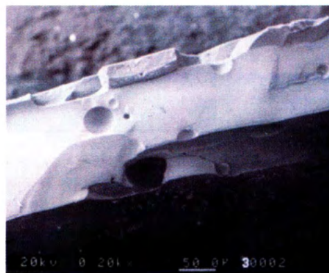
Fig. 10 - SEM Micrograph of gel layers on enamel.
