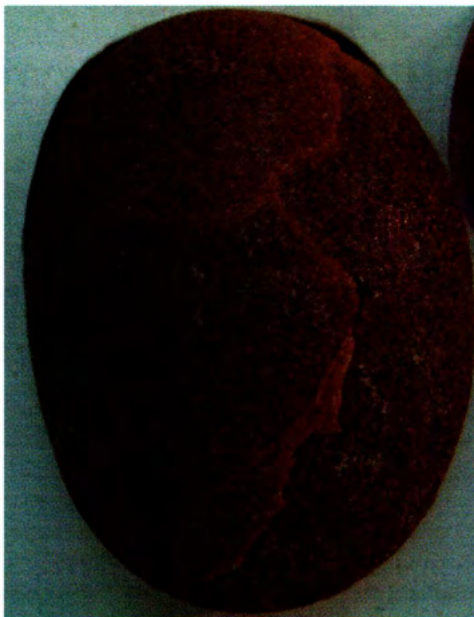
Fig. 5 - Damage to amber surface after approximately one hundred years around 75% RH.
