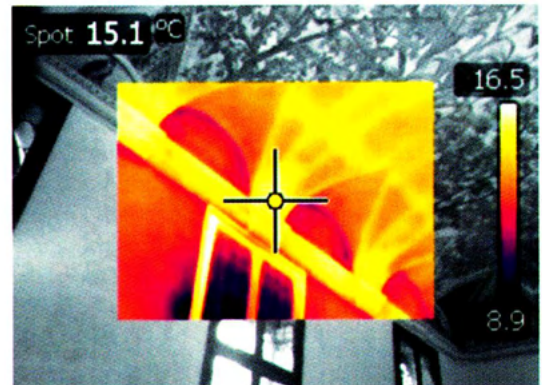
Fig. 7 - Structural discontinuities made visible in a thermal image. Yellow indicates the warmest surfaces, e.g. the wooden frame of the window, the cornice in stucco just below the vaulted ceiling, the wooden frames supporting the vaults. Orange is also warm, but less than yellow. Blue indicates the coldest surfaces, i.e. the window panes and the wall adjacent to the window opening. Violet is an intermediate cold level, e.g. between orange and blue, or typical of the areas hardly reached by warm air motions, e.g. the borders of the lunettes, the edge between the cornice and the wall.
