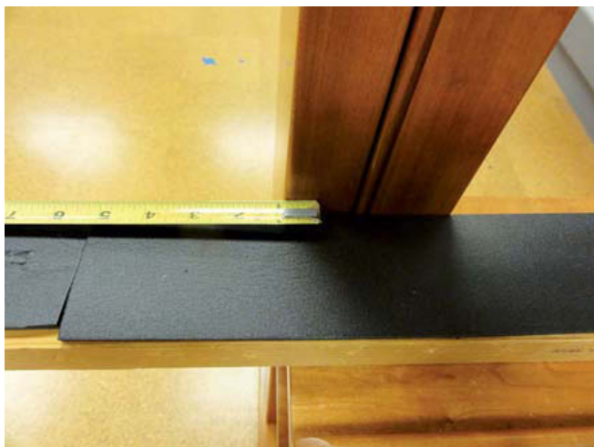
Fig. 3 – The easel will cover approximately \frac{3}{4} inches of the vertical stretcher bars. Lock wheels on each easel.
