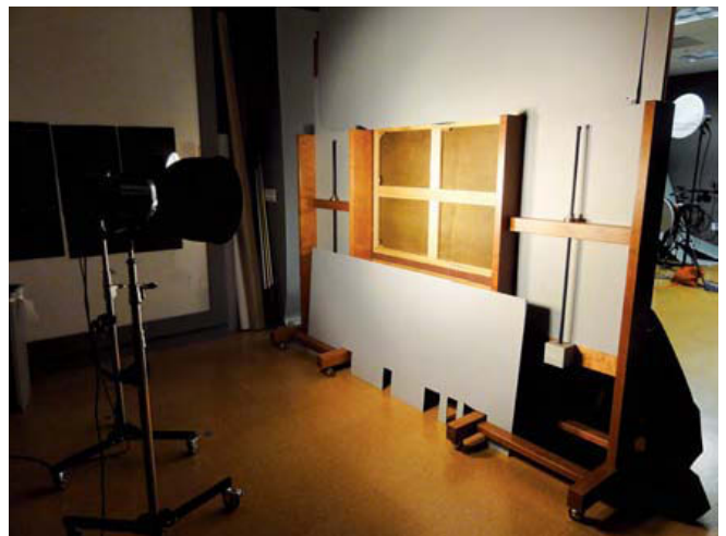
Fig. 14 – Place lights behind the painting at a distance, about three feet.
