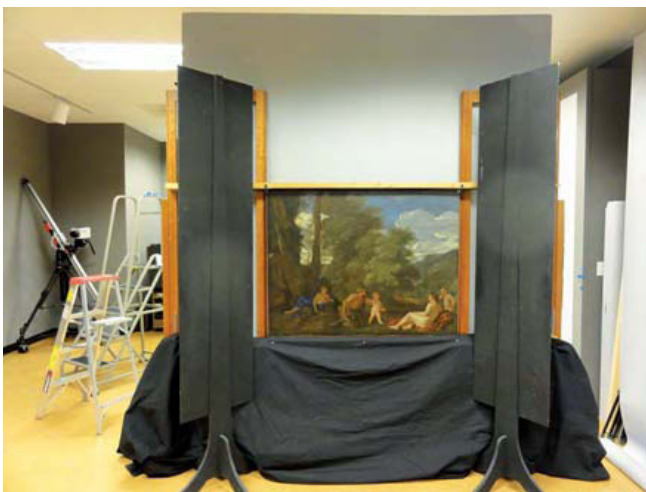
Fig. 13 – Block out stands are also used to obstruct unwanted light.
