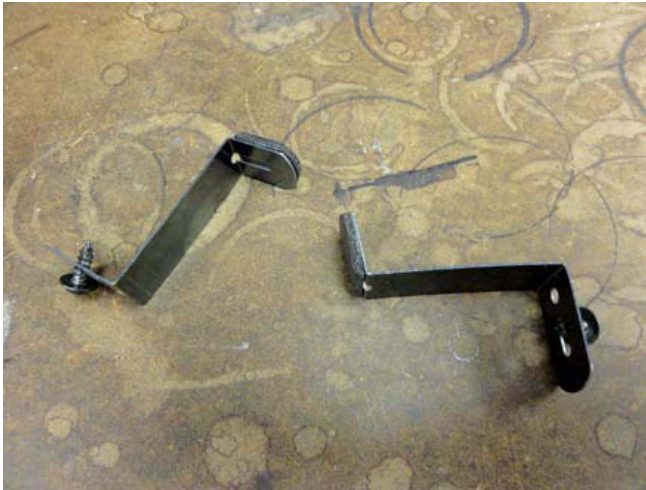
Fig. 9 – While one person holds the painting in place, another measures the distance from the painting surface to the front edge of the top 2 x 4. This distance will be needed to bend the padded mending plates into a Z shape.
