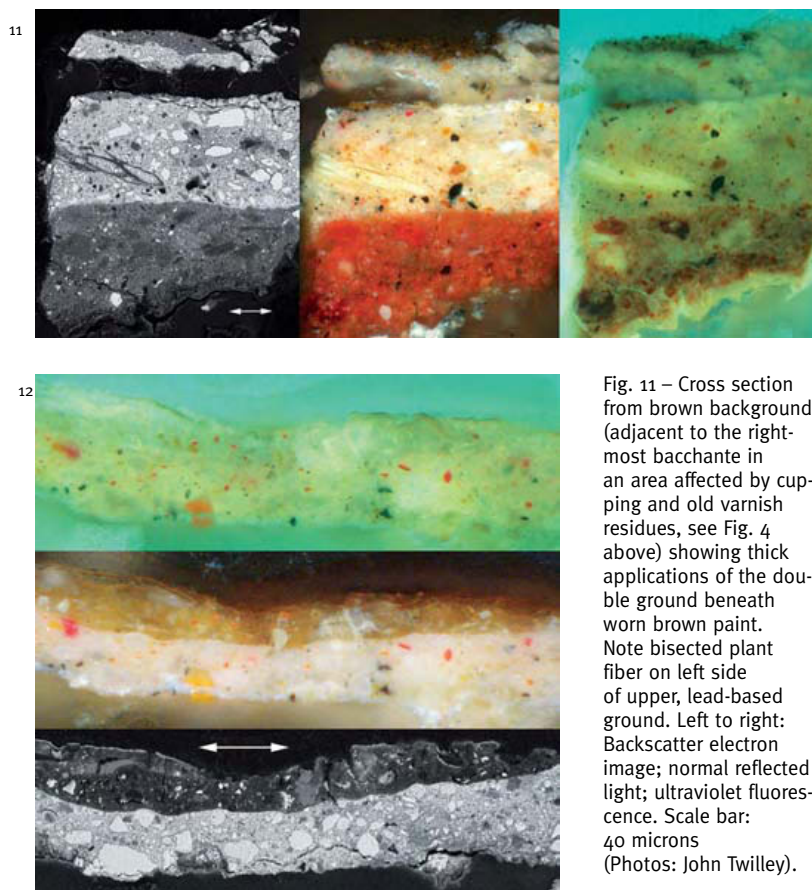
Fig. 12 – Cross section of the pink scarf of the rightmost bacchante with a sequence of three layers starting with the upper ground. A thin layer of lake pigment, most visible at the left end of the sample, was applied atop the light brown paint surrounding the figure. Its upper surface bears a coating of lead compounds visible as a light band in the SEM view. Top to bottom: ultraviolet fluorescence, normal reflected light, backscatter electron image. Scale bar: 40 microns (Photos: John Twilley).
