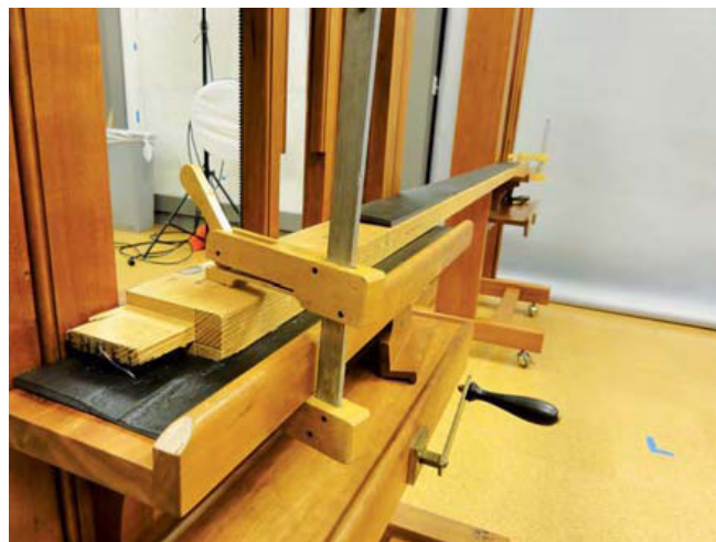
Fig. 4 – Clamp one 2 x 4 to the lower bottom tray shelves of the easels.
