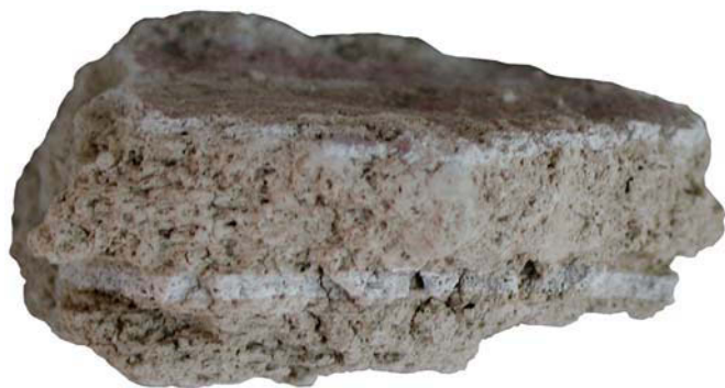
Fig. 25 – inv. 8048, showing a double stratification for the mud plaster and the top final gypsum coating.
