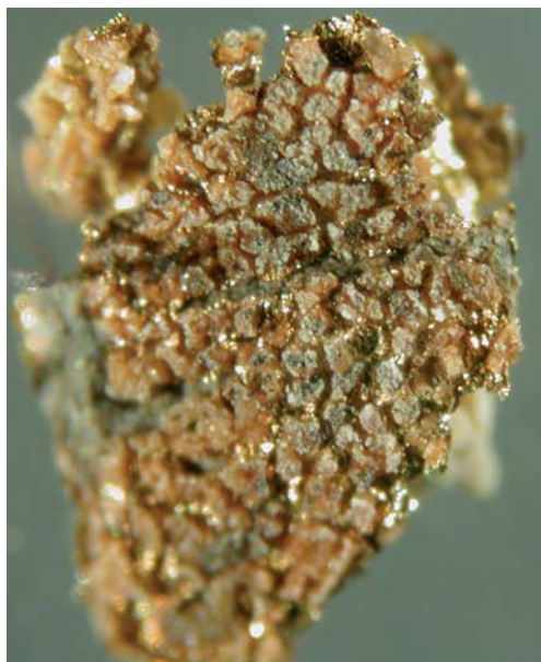
Figs. 44-45 – sample 3. The fragment photographed before the embedding in polyester resin. The surface-looking side (44) shows some varnish residues over the gold foil. The rear side (45) shows the oil-resin mordant.
