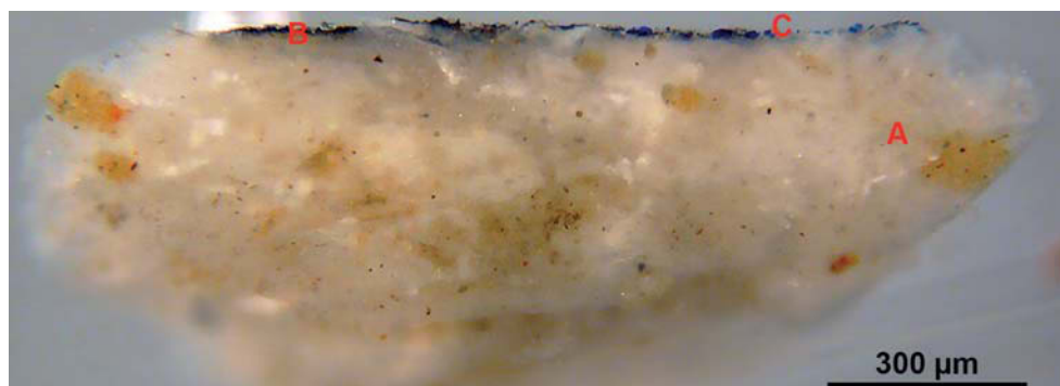
Fig. 22 – sample 4. Cross-section showing the ground-layer (A) interspersed with yellow masses of possible proteinaceous substances. The upper layer (C) consists of ultramarine blue obtained from lapis lazuli (photo CSG Palladio).
