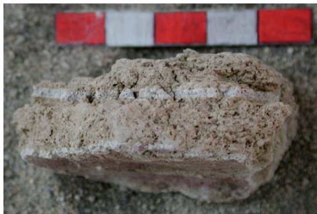
Fig. 61 – inv. 8048, side view. Fragment showing two distinct layers. The re-decoration had been carried out on a new mud plaster and a new fine gypsum coating.
