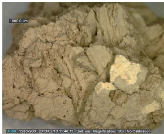
Fig. 19 – detail of the back of sample 3, with the mud plaster filled with straw ( kähgil ) on view.
