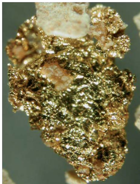
Figs. 44-45 – sample 3. The fragment photographed before the embedding in polyester resin. The surface-looking side (44) shows some varnish residues over the gold foil. The rear side (45) shows the oil-resin mordant.
