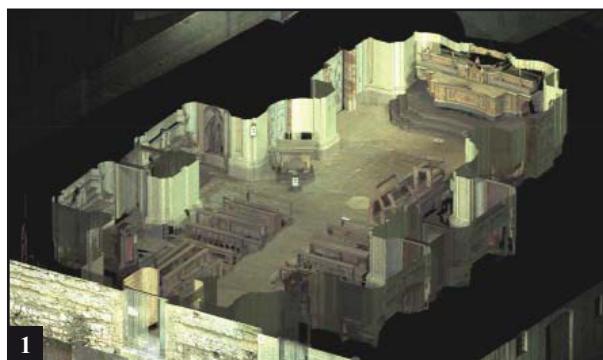
Fig.1 – Point cloud display in half space of the San Filippo Church at Cagli
