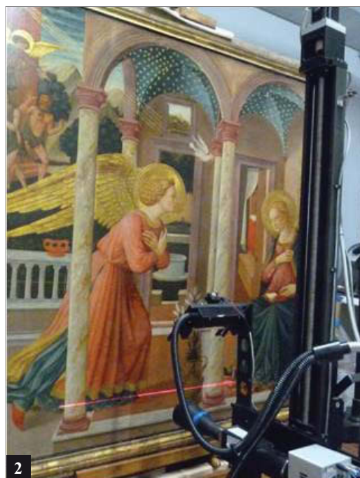
Fig. 2 - IFAC-CNR HSI prototype scanner during data acquisition.
