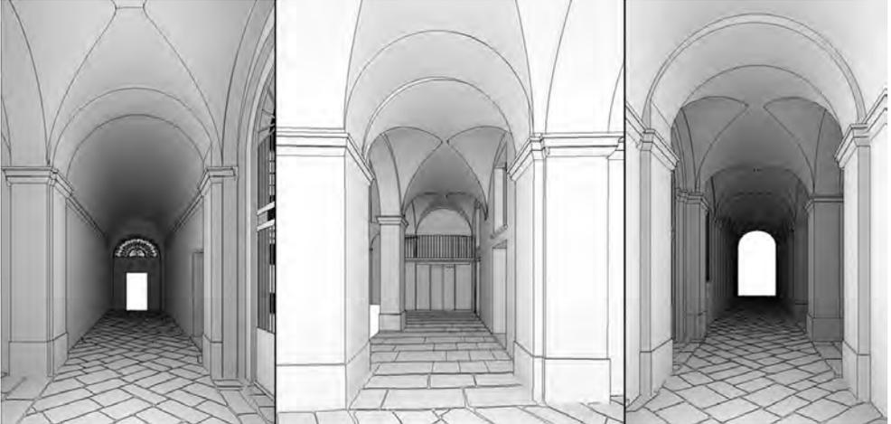
Fig. 4 - Representation of the vaulted system of the hallway, from right: barrel vault of the entrance on Via Porta Pretoria; cross vaults of the inner courtyard; cross vaults with different spans of the entrance on Piazza Plouves.
