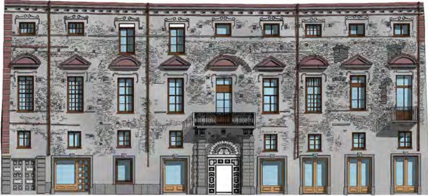
Fig. 2 - North elevation of Palazzo Ansermin in BIM environment.
