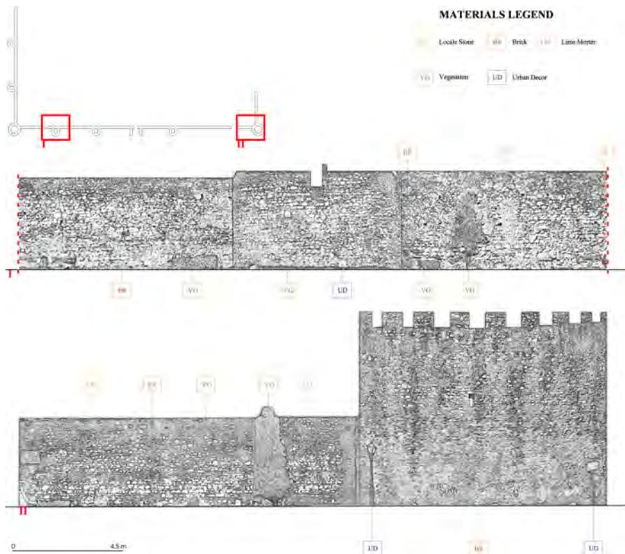
Fig. 5 - The Elbasan Fortress. Material survey of wall portions.
