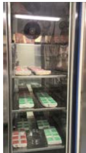
Figura 14. Mattoni in cella climatica (Angelantoni, mod. Challenge 5000).
