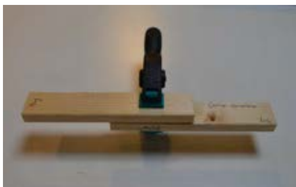
Figura 5. Provino “single lap”
